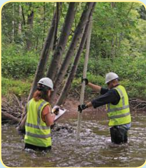
Figure 3 - Measuring stream morphology changes around a LWD structure
